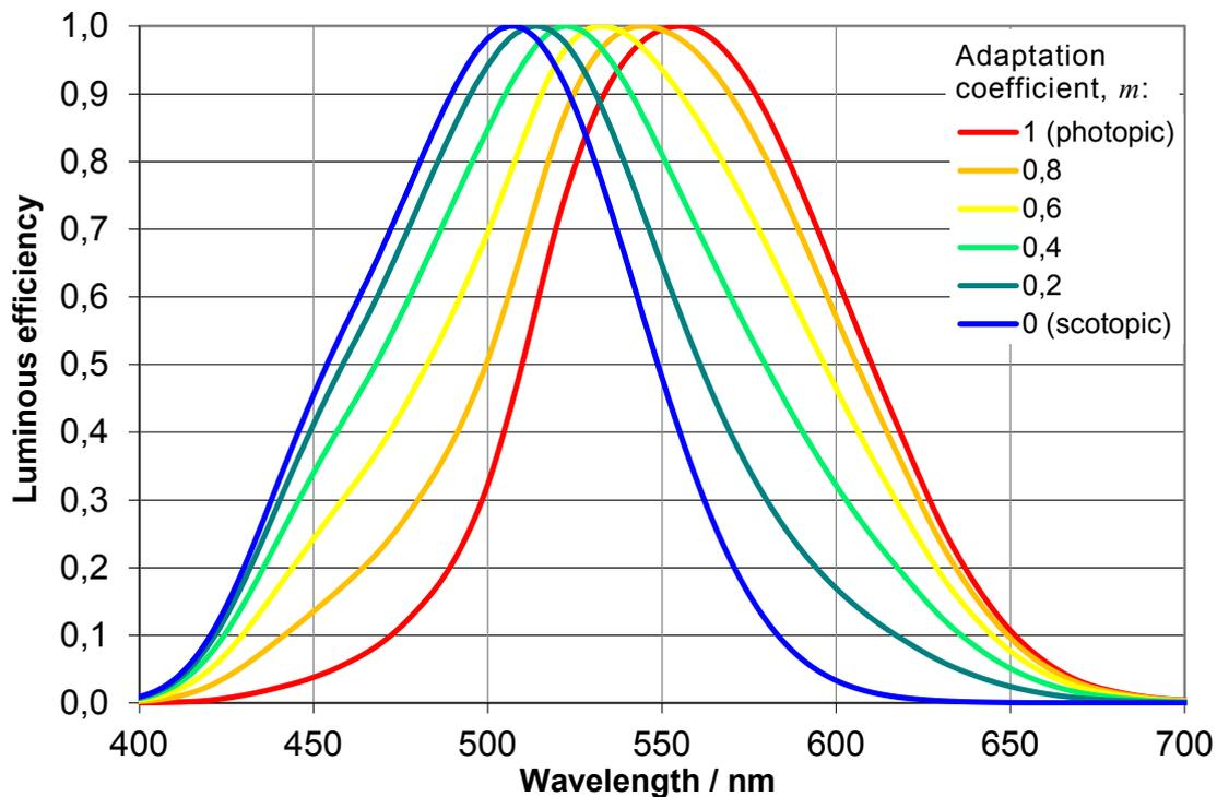
**Figure 1 – Spectral luminous efficiency functions  $V_{\text{mes};m}(\lambda)$  for various values of the adaptation coefficient,  $m$**
